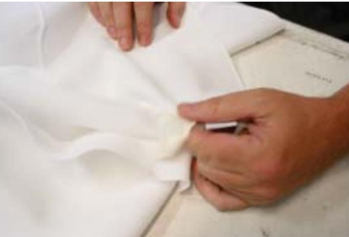
The RFID chip is sewed into a 2-inch by 2-inch piece of fabric on the back of the table linen.
