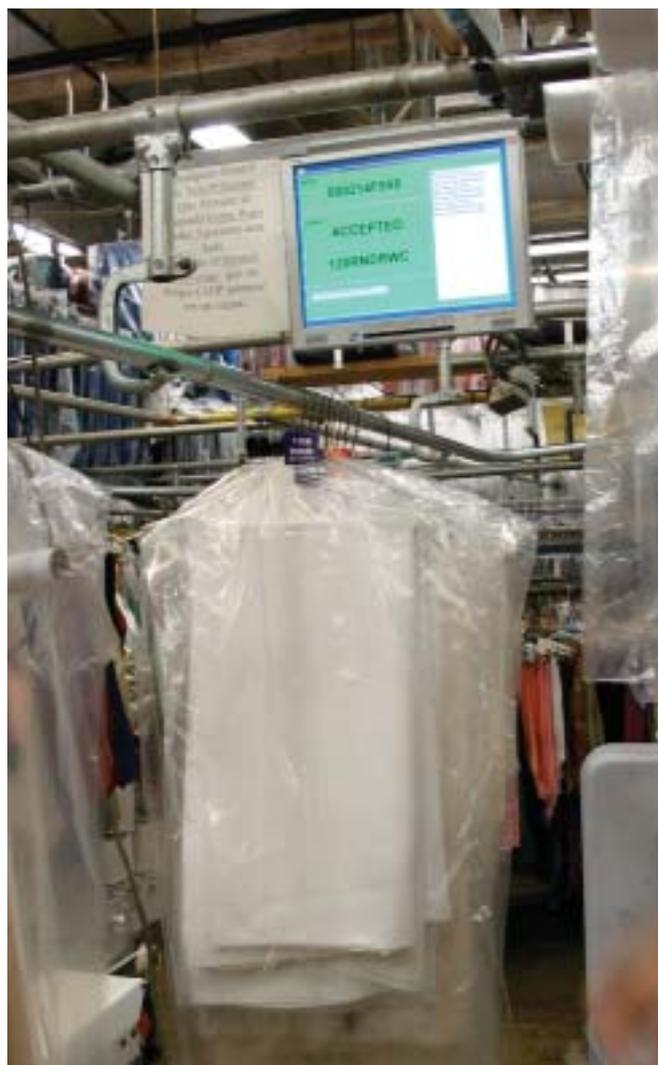
Table linen inventory is sorted by using man-readable, color-coded tags indicating the item's size as well as an RFID tag.
